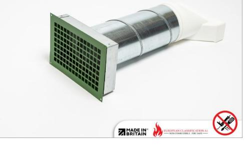
Rytons A1® Fire-rated Ducting Kit 125mm Dia. with Square Holed Double Air Brick Flanged Custom RAL colour air brick in matt, semi-gloss or gloss finish achieving Class A2-s1, d0 RAL6010 (Grass green) matt finish pictured Connector for 204mm x 60mm ducting Registered Design 6109951 Patent Approved Product Code: A1DK125SQDF
